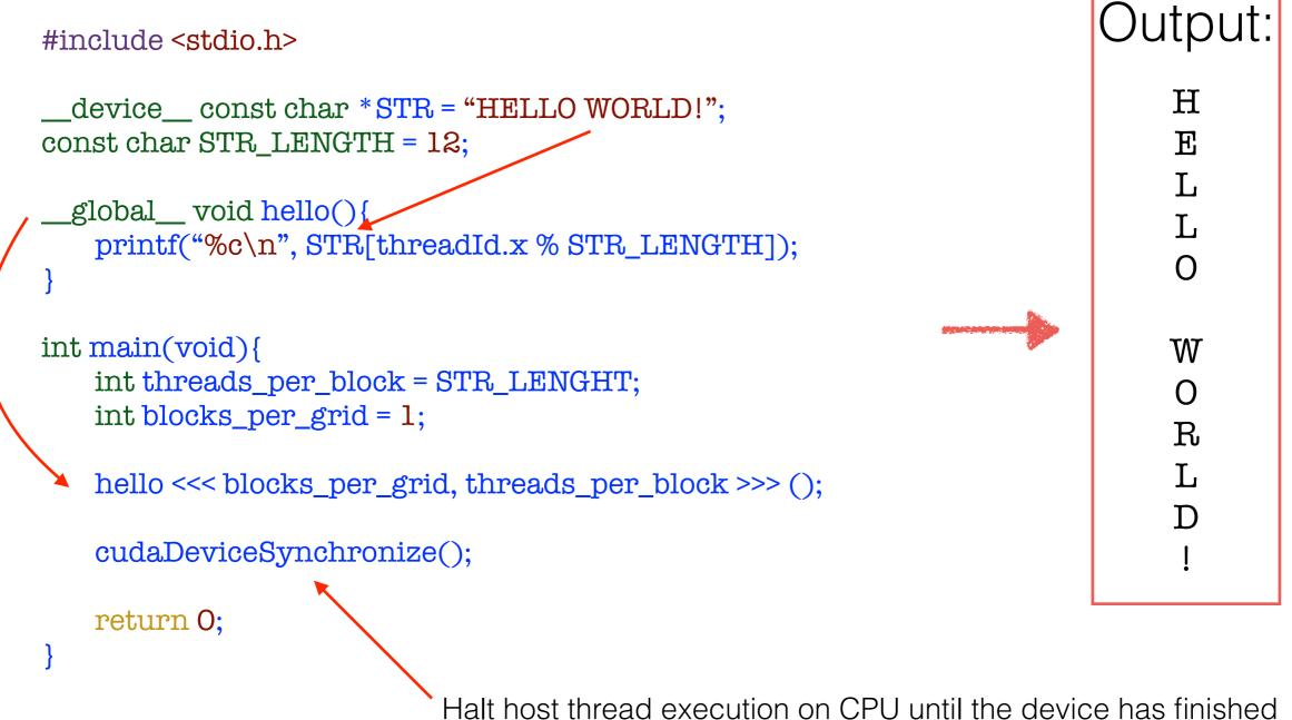
Palt host thread execution on CPU until the device has finish processing all previously requested tasks.
